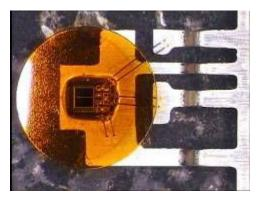
Figure 2. Reinforcing Critical Functional Pads with Double Wire Bonds
