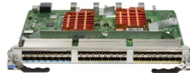
48-port Gen 6 Brocade FC32-48 port blade with 32G line rate performance
