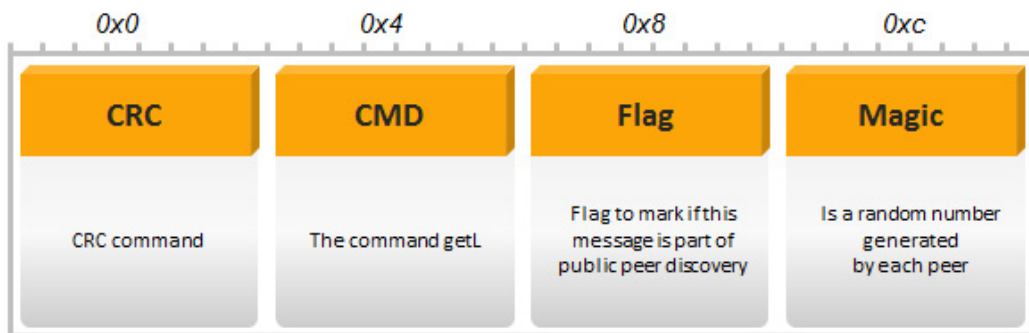
Figure 18. Version 2 response to getL command structure
