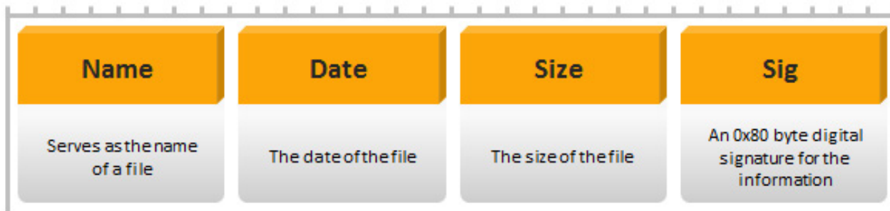
Figure 23. retL command structure
