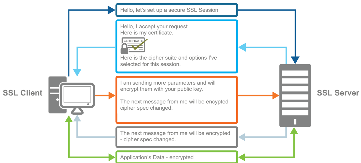
Figure 2 – Illustrates the Sequence of SSL transactions
