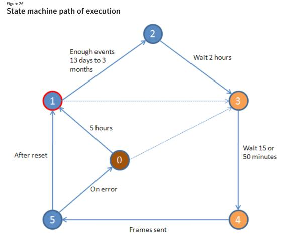
In states 3 and 4 two network send bursts occur. The traffic generated is semi-fixed, and can be one of the two sequences. The sequences consist of multiple frames that each contain 31 records. Each frame is sent to each CP 342-5 module, which passes on the respective record within the frame to each of the 31 frequency converter drive slaves.
