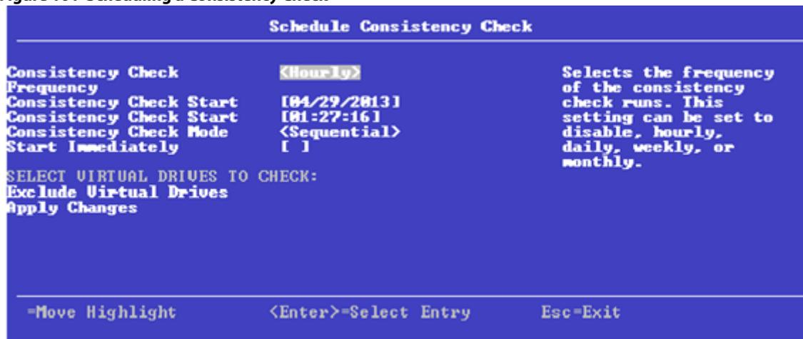
2. Select the desired interval at which to run consistency checks.
