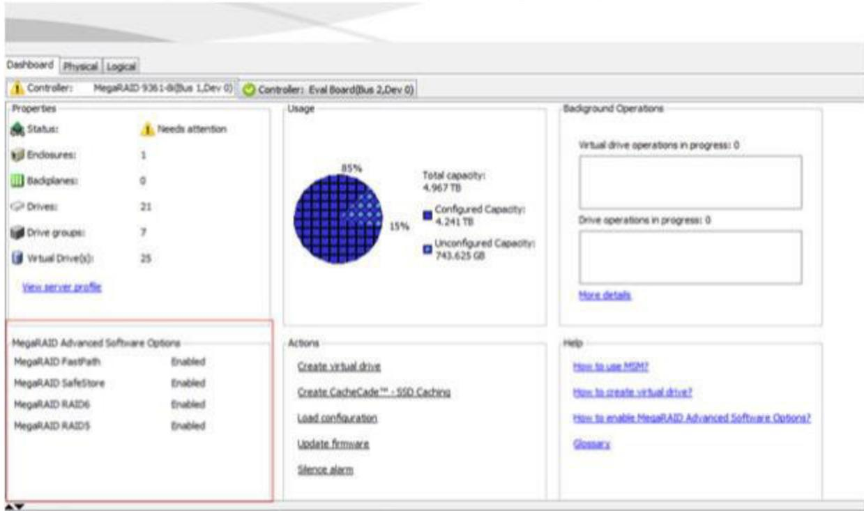
Figure 234 Manage MegaRAID Advanced Software Options Dialog
