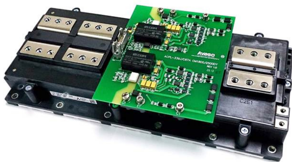
Figure 1. Mitsubishi IGBT CM1800DY with ACPL-339J and ACPL-C87A gate drive reference board
