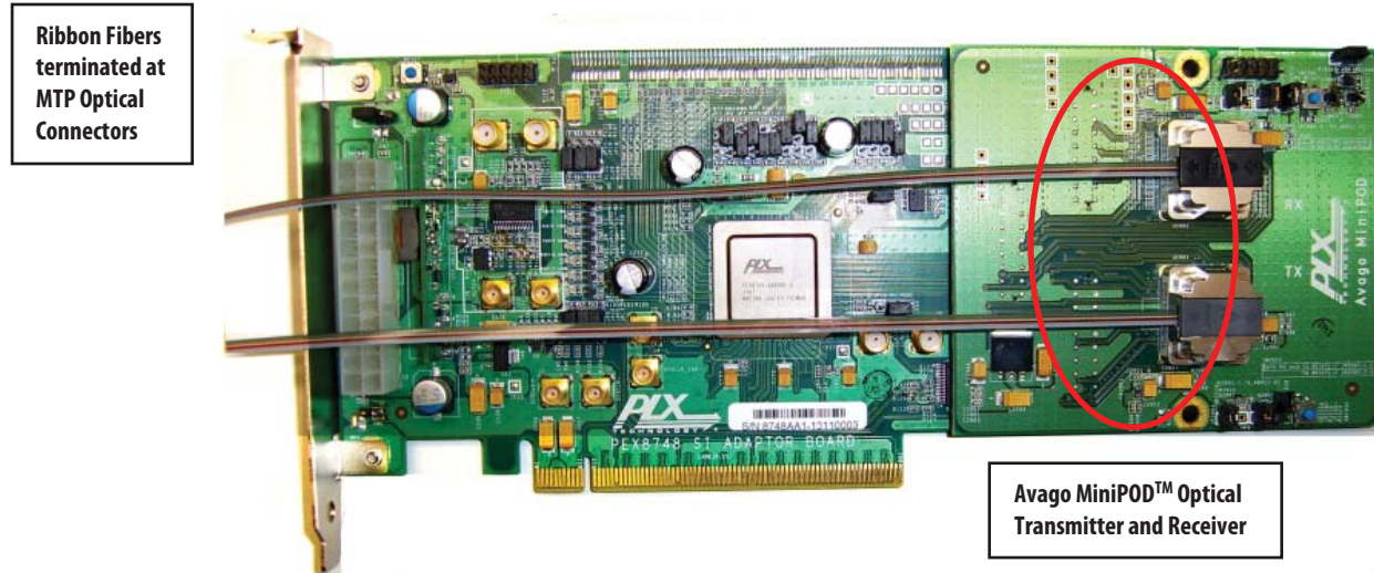
Figure 2. PEX8748 SI card with Avago Technologies MiniPOD™ adapter
