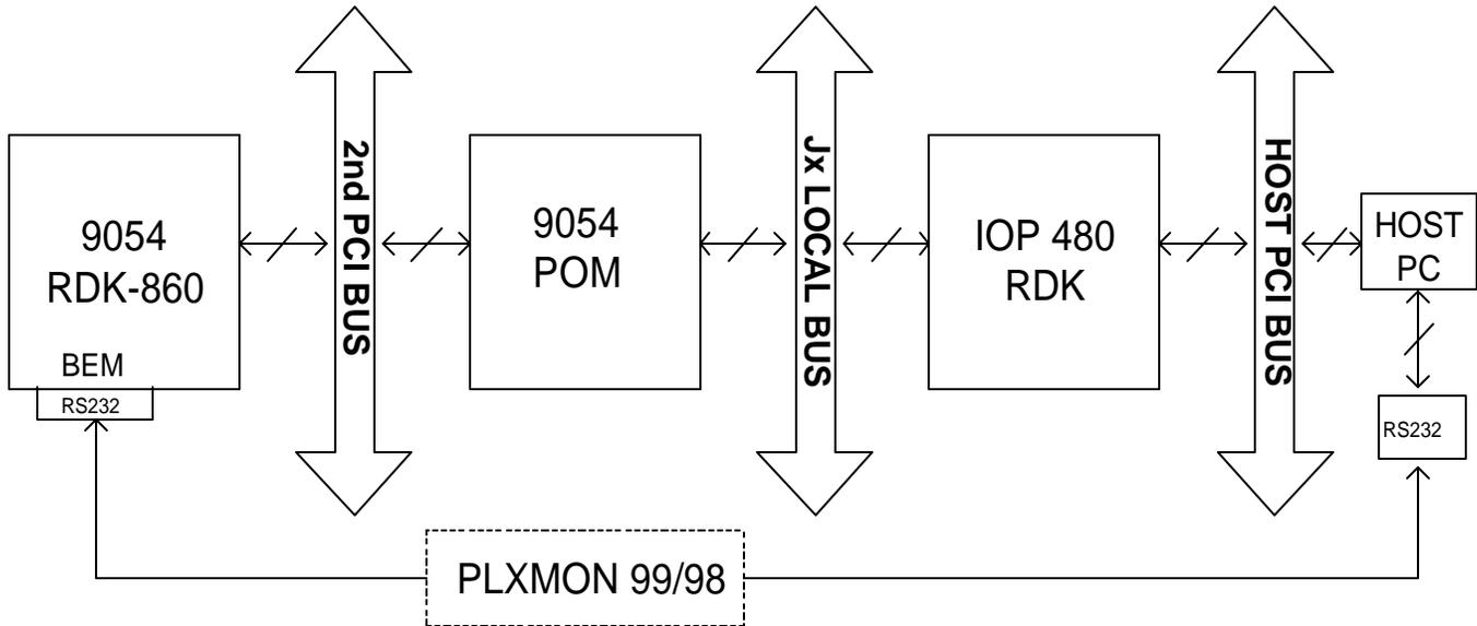
**Figure 1. PCI 9054 POM1 Application Block Diagram**
