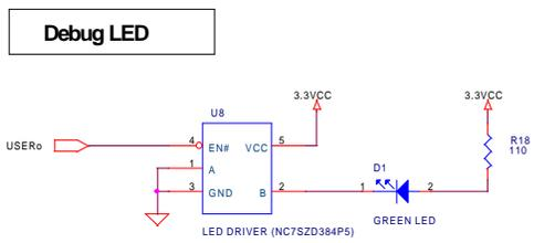
Place 0.1 uF as close to the VCC pin of LED driver as possible.
