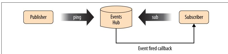
*Figure 5-5. Asynchronous message-passing implemented with a PubSubHubbub-inspired flow*
