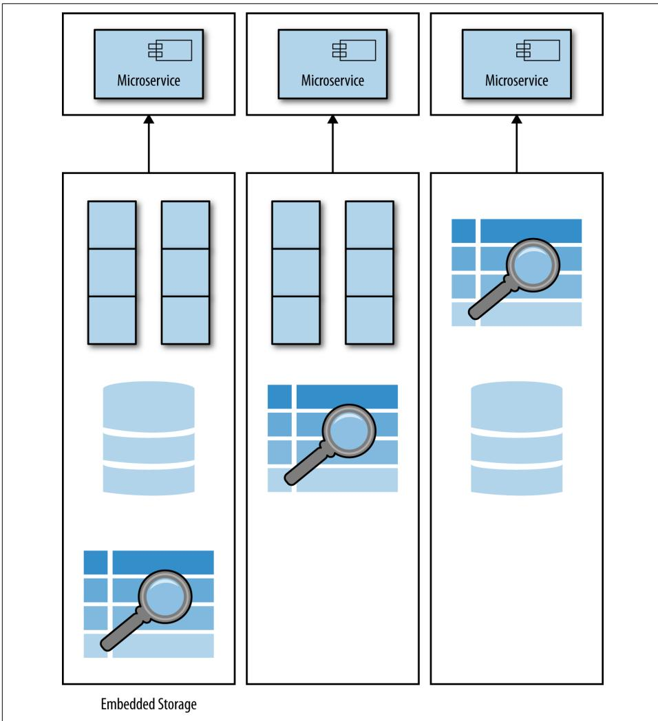
*Figure 5-7. Components using fully embedded, isolated dependencies*
