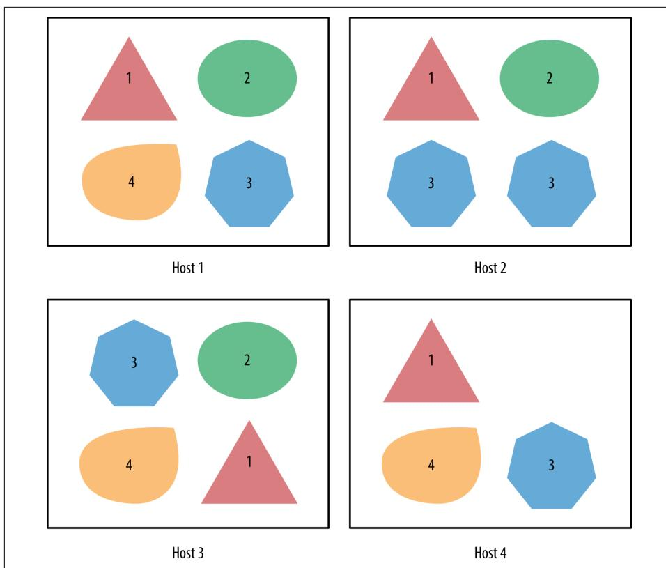
Figure 6-1. Microservice deployment topology with nonuniform service distribution
