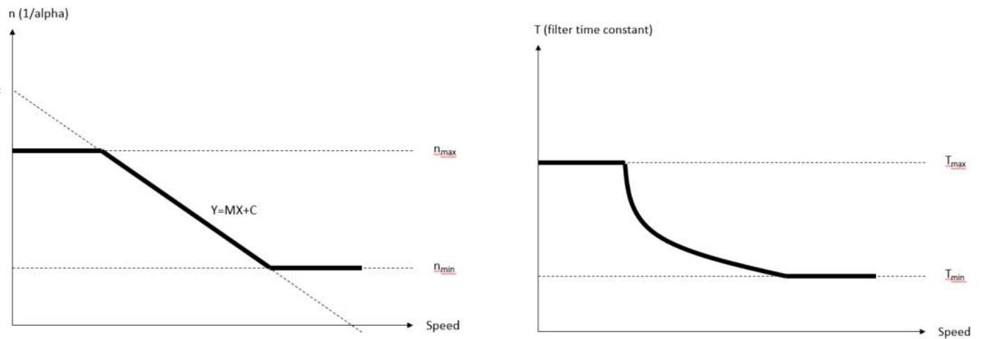
By default, the dynamic filter is enabled, with a maximum filter time constant ( $T_{max}$ ) of 1.5 ms when the speed is <300 rpm and a minimum time constant ( $T_{min}$ ) of 1.3 ms when the speed is >500 rpm.
