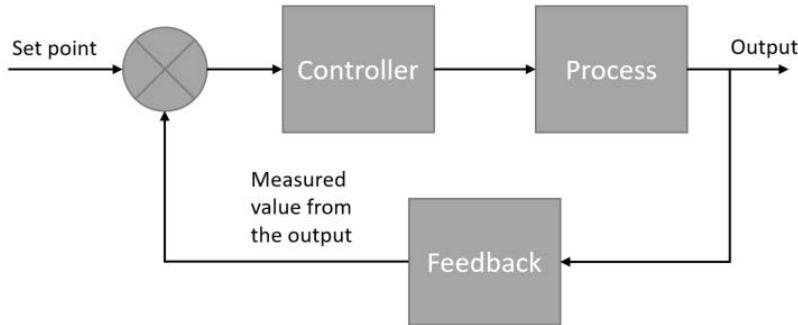
A closed-loop system is formed by three components: controller, process, and feedback:
