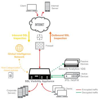
Figure 1 - The Symantec SSL Visibility Appliance deployed within a network
