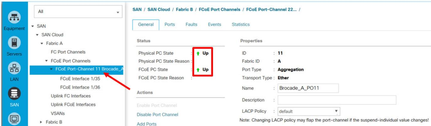
Perform the same steps to verify that the FCoE port channel is connected to Fabric-B.
