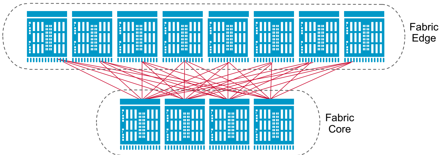
Figure 1: Twelve-Chassis Core/Edge Topology Supported with the Brocade X7, X6, and/or DCX 8510
