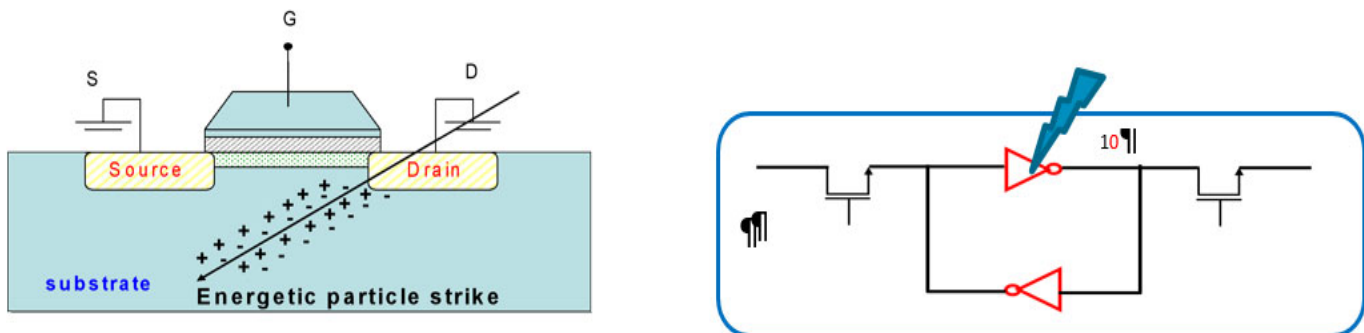
Figure 1: Silicon Transistor during Energy Particle Strike
