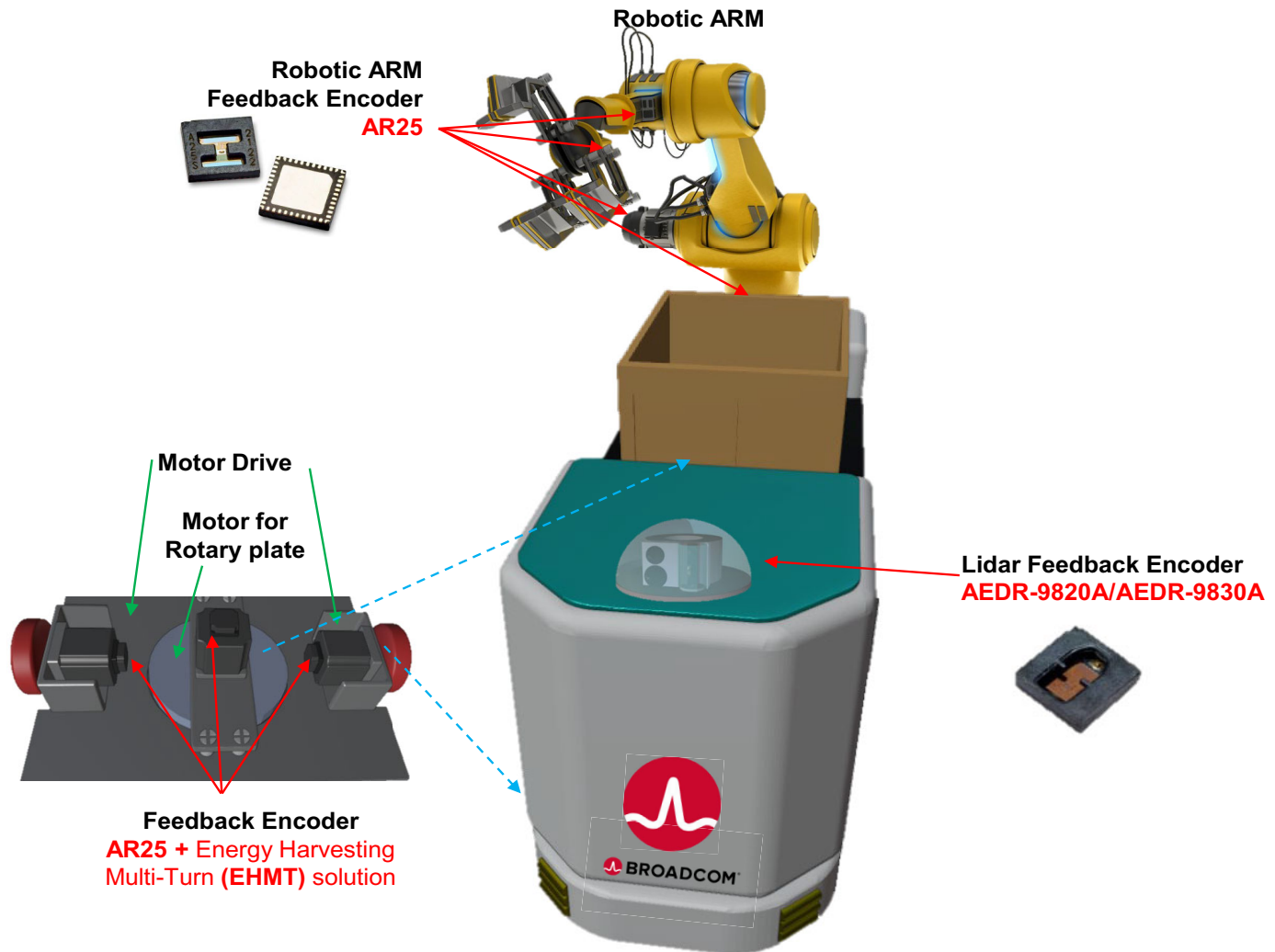
Figure 1: Autonomous Guided Vehicle/Mobile Robot Integrated with Broadcom Encoders
