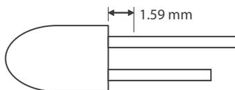
Soldering the LED using a soldering iron tip closer than 1.59 mm might damage the LED.
