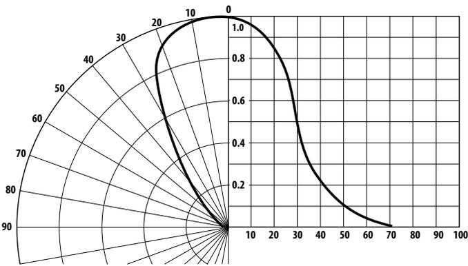
**Figure 9: Relative Luminous Intensity vs. Angular Displacement for T-1¼ Package**
