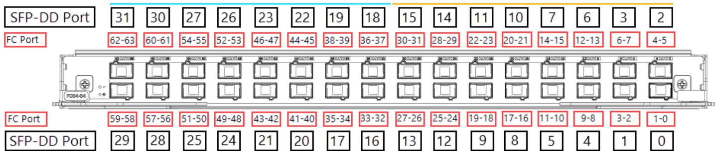
Figure 4: Brocade FC64-64 Port Blade Port Numbering
