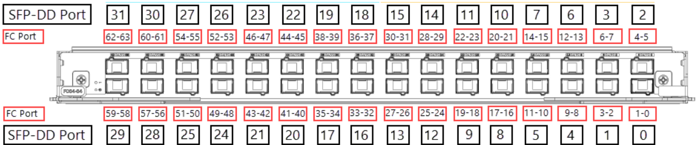
Figure 3: Brocade FC64-64 Port Blade Port Numbering
