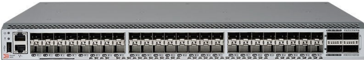
Figure 4: Brocade G620 Switch with 4 x Q-Flex MPO Connectors
