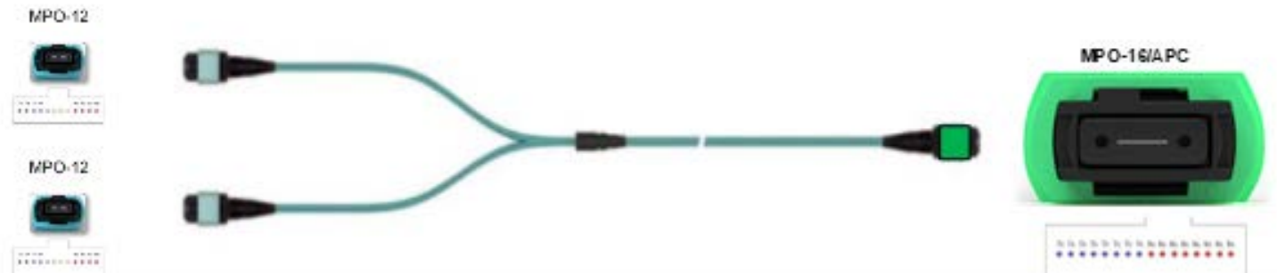
Figure 17: Gen 7 to Gen 8 ICL Connectivity using MPO-16/APC to 2x MPO-12/UPC Y-cable
