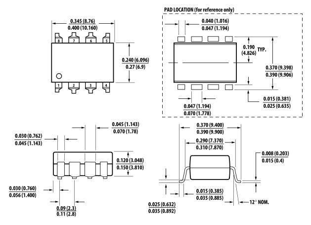
DIMENSIONS INCHES (MILLIMETERS)  $\frac{\text{MIN}}{\text{MAX}}$ LEAD COPLANARITY = 0.004 INCHES (0.10 mm)
