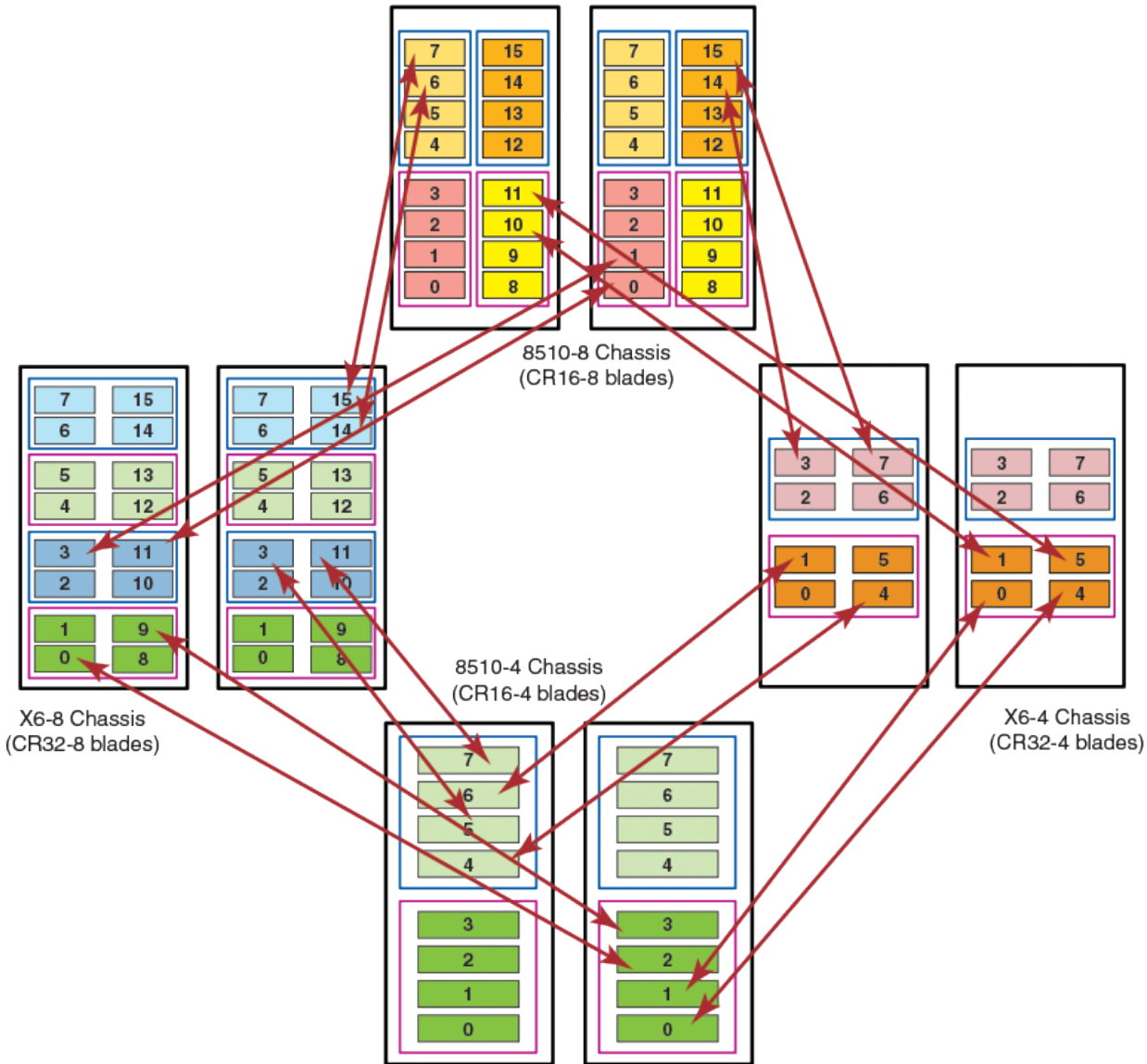
Figure 36: ICL Trunks between DCX 8510 Backbones and X6 Directors
