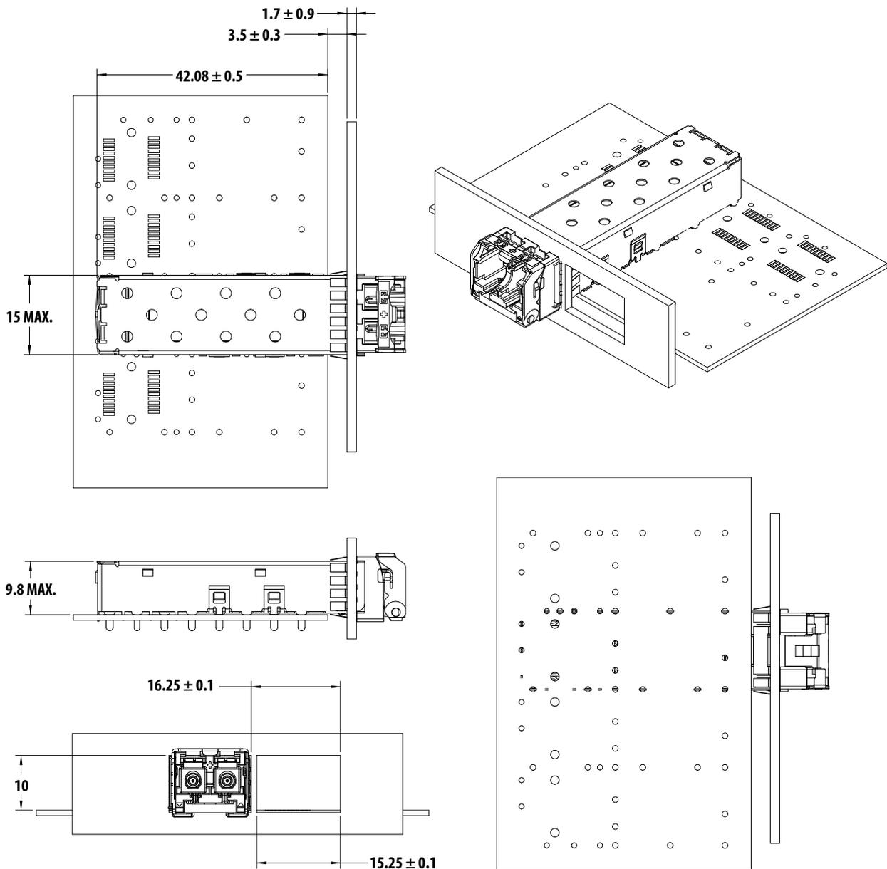
Figure 8. SFP Assembly drawing
