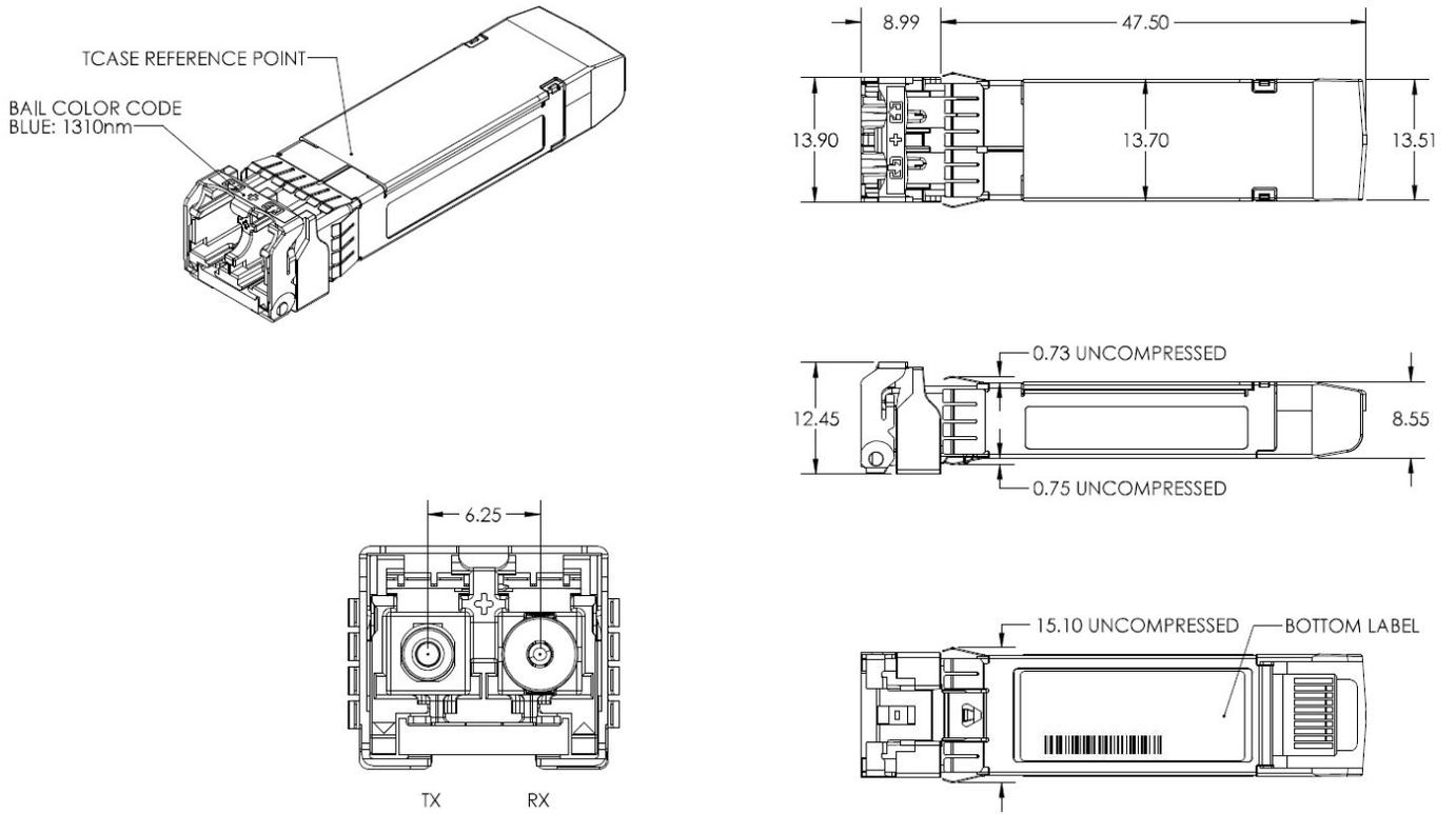
Figure 5. Module drawing
