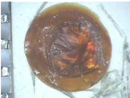
Figure 10 The Polyimide Film of the ACPL-337J After Direct Current Injection Test
