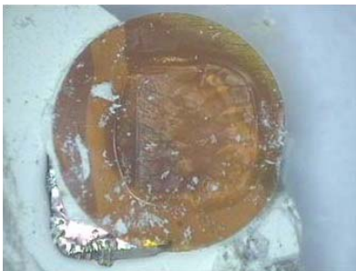
Figure 5 The Polyimide Film of the ACPL-337J After Short Circuit Test
