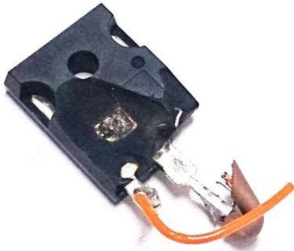
Figure 4 The Destruction of the IGBT After Short Circuit Test
