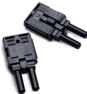
Figure 11. Duplex versatile link connector attaches the first section of the wiring to the optical sensor transceiver
