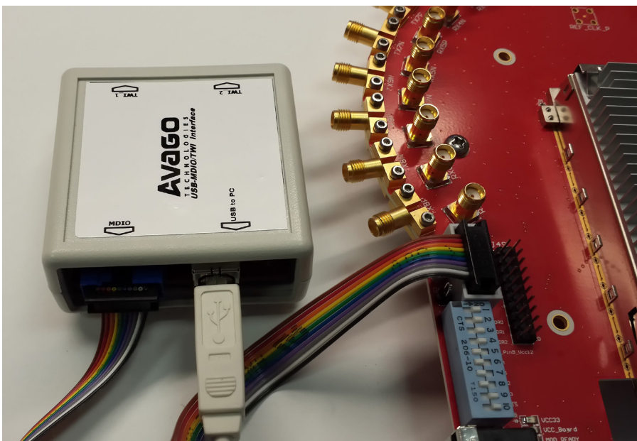
Figure 7. Avago Technologies USB-MDIO controller connection to CFP2 evaluation board
