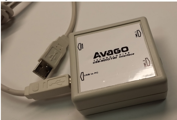
Figure 6. Avago Technologies USB-MDIO Controller – USB for power; MDIO communication
