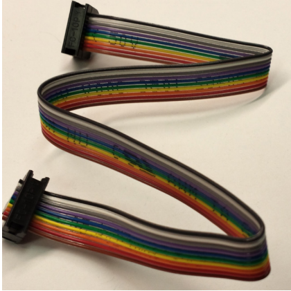
Figure 5. Ribbon Cable for MDIO-to-CFP2 Evaluation Board Connection
