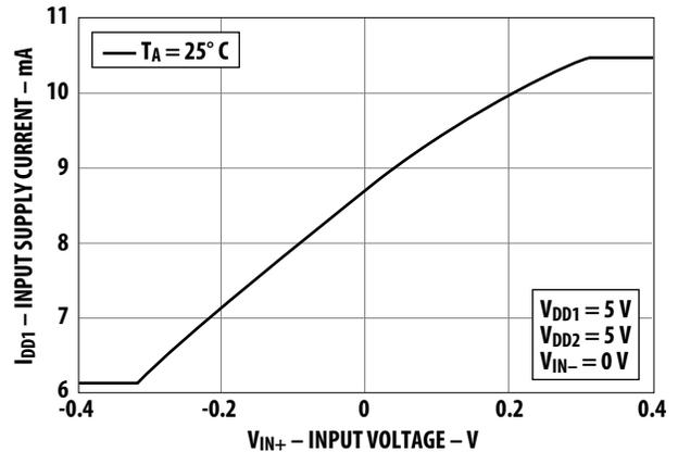
Figure 15 Output Supply Current vs. Input Voltage
