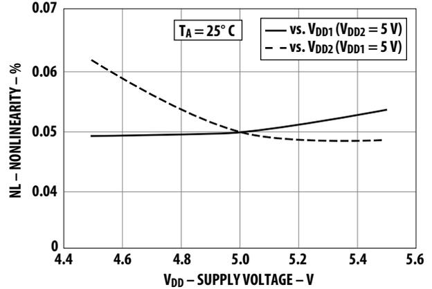
Figure 11 100-mV Nonlinearity vs.  $V_{DD1}$  and  $V_{DD2}$
