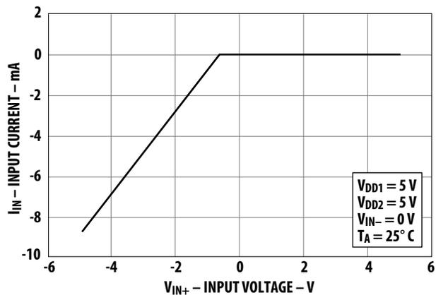
Figure 14 Input Supply Current vs. Input Voltage
