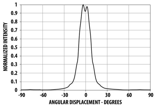
Figure 8: Representative Radiation Pattern for 23° Viewing Angle Lamp
