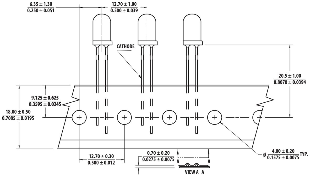
**NOTE:** The ammo-packs drawing is applicable for packaging option -DD and -ZZ and regardless standoff or non-standoff.
