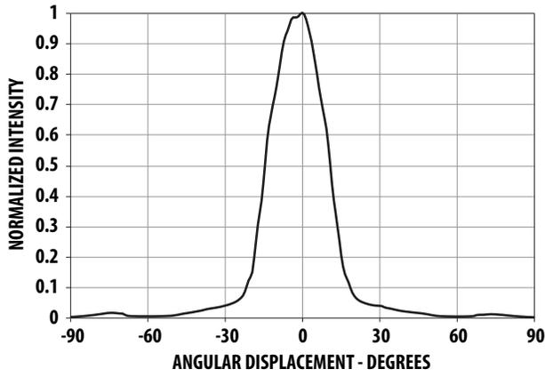
Figure 9: Representative Radiation Pattern for 30° Viewing Angle Lamp
