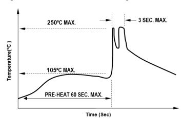
**NOTE:** Figure 21 refers to measurements with thermocouple mounted at the bottom of the PCB.
