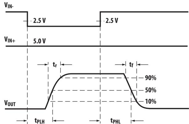
Figure 54.  $V_{OUT}$  propagation delay waveforms, inverting configuration.
