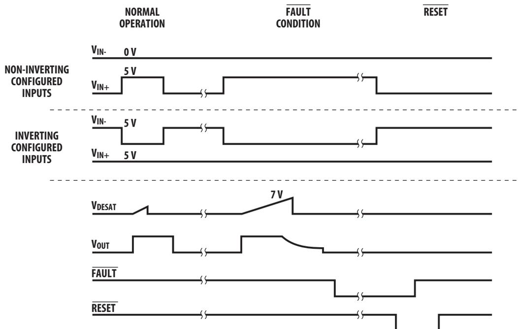
Figure 62. Timing diagram.
