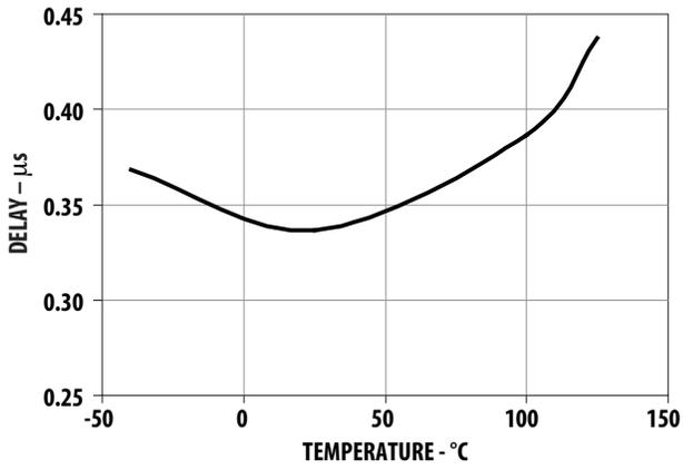
Figure 23. DESAT sense to 90% Vout delay vs. temperature.
