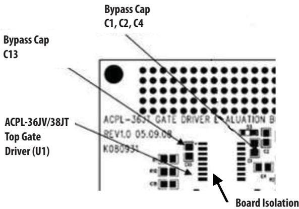
Figure 77a. Bypass Capacitors
