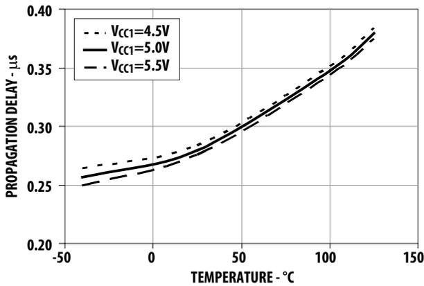
Figure 19.  $V_{IN}$  to high propagation delay vs. temperature.
