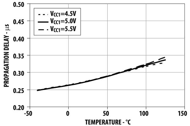
Figure 20.  $V_{IN}$  to low propagation delay vs. temperature.
