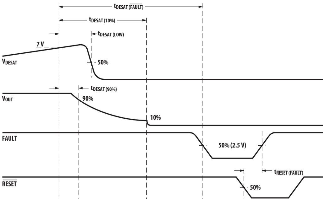
Figure 55. Desat,  $V_{OUT}$ , fault, reset delay waveforms.
