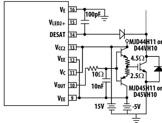
Figure 74. Current buffer for increased drive current
