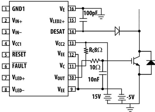
Figure 73. Use of RC to further limit  $I_{ON,PEAK}$ .
