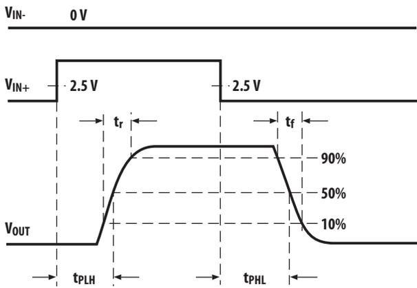
Figure 53.  $V_{OUT}$  propagation delay waveforms, noninverting configuration.
