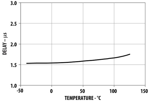
Figure 24. DESAT sense to 10% Vout delay vs. temperature.
