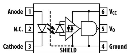
Note: A 0.1  $\mu$ F bypass capacitor must be connected between pins 4 and 6.
