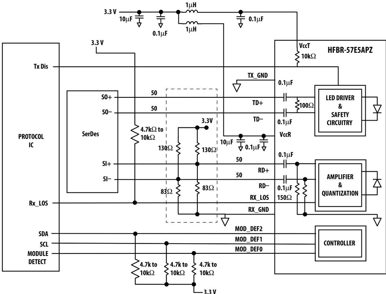
**Figure 6. Avago Technologies' HFBR-57E5APZ Fast Ethernet Fiber Optic Transceiver Driving Circuitry**
