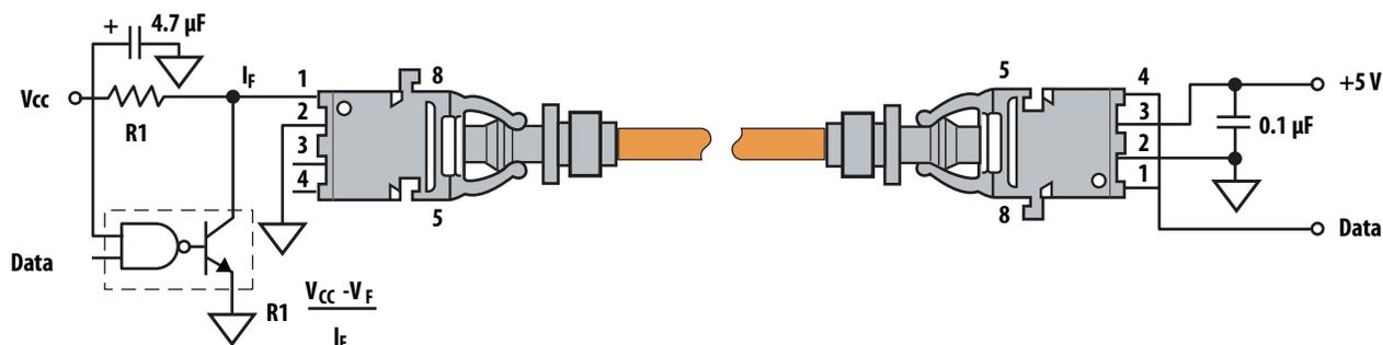
Figure 3. HFBR-1521Z/2521Z Circuit Diagram for 5MBd Data Rate
