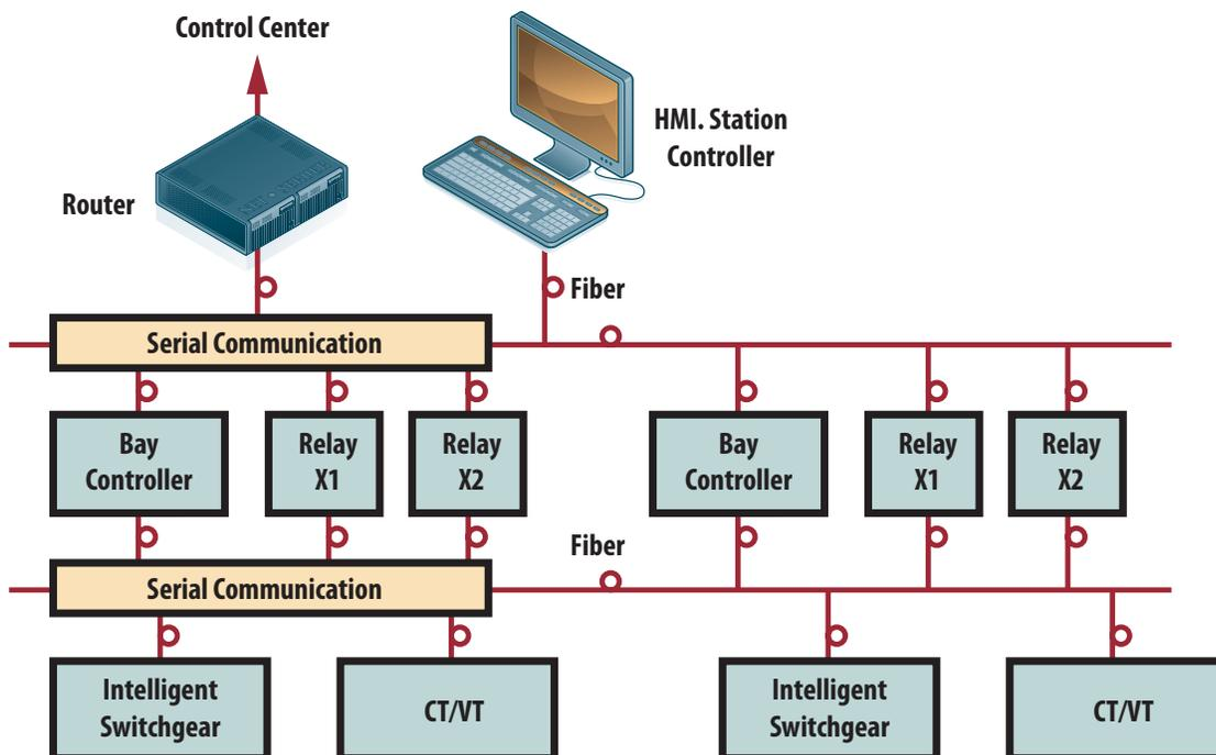
Figure 5. Substation Automation based on IEC 61850
