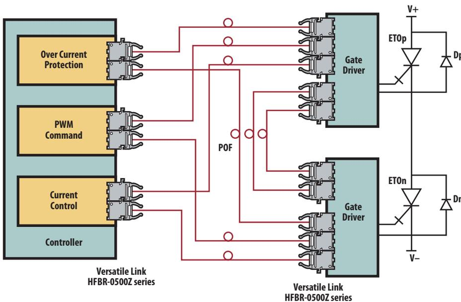
Figure 3. ETO Two-Level Voltage Source Converter Phase Leg Block Diagram
