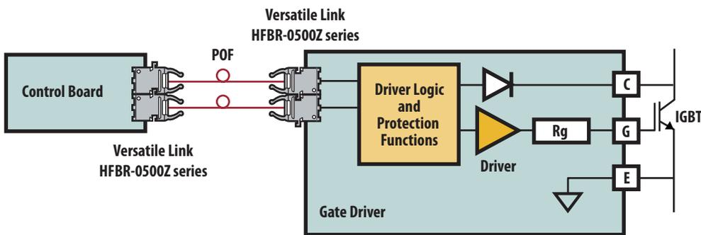
Figure 2. IGBT Gate Driver Block Diagram
