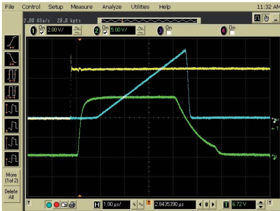
Figure 6. Channel 1 (Yellow) – Input LED, Channel 2 (Green) – Output Voltage, Channel 3 (Blue) – DESAT
