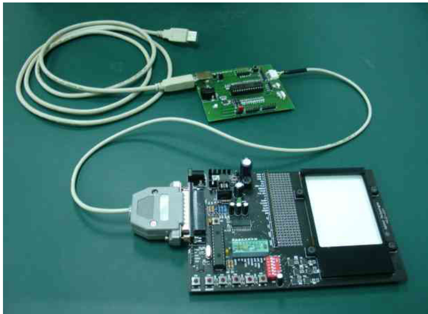
Figure 4. Setup connection for USB-2-I2C with HDJD-JD11
