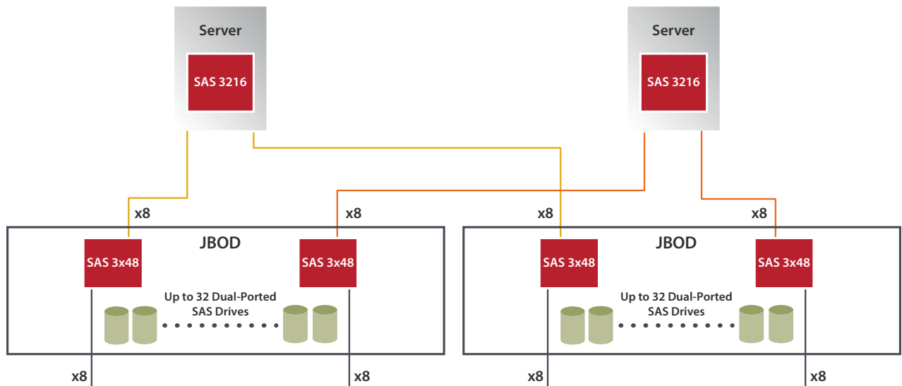
Figure 3: SAS 3216 Topology Diagram
