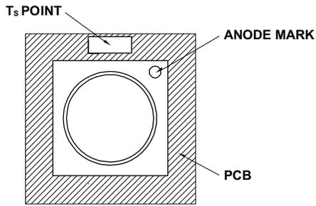
$T_S$  can be easily measured by mounting a thermocouple on the soldering joint as shown in preceding figure, while  $R_{\theta J-S}$  is provided in the data sheet. Verify the  $T_S$  of the LED in the final product to ensure that the LEDs are operating within all maximum ratings stated in the data sheet.
