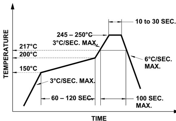
Figure 15: Recommended Board Reflow Direction
