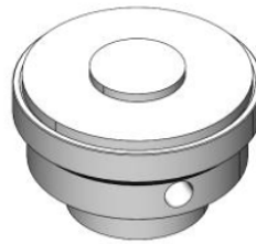
Figure 5: Modulation Element 12-mm × 2-mm Neodymium Magnet Mounted in an Aluminium Hub
