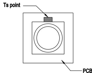
$T_S$  can be easily measured by mounting a thermocouple on the soldering joint as shown in [Figure 17](#), while  $R_{\theta J-S}$  is provided in the data sheet. Verify the  $T_S$  of the LED in the final product to ensure that the LEDs are operating within all maximum ratings stated in the data sheet.
