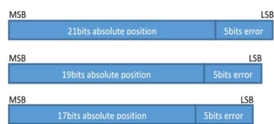
Figure 12: AR18 SSI 3-Wire Format Output
