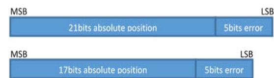
Figure 13: AR35 SSI 3-Wire Format Output
