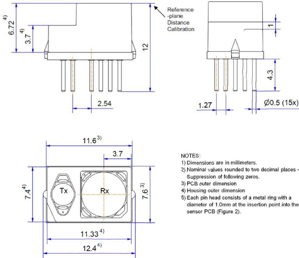
Figure 2: Module Bottom View (Dimensions in mm)
