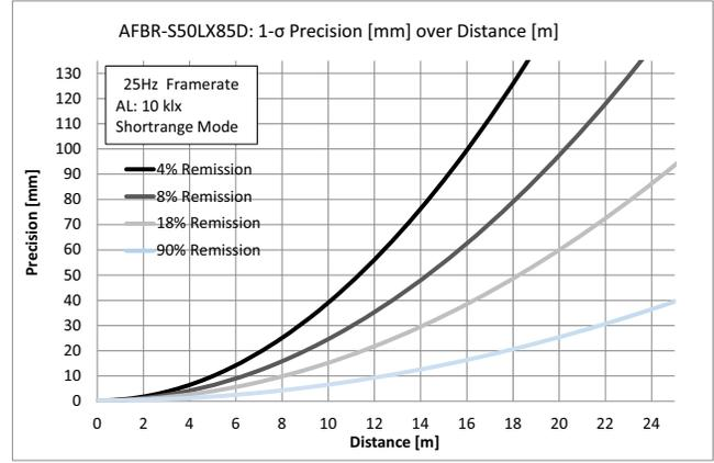
**Figure 10: Typical Precision [mm] over Distance [m] – 50 klx, Short Range Mode**
