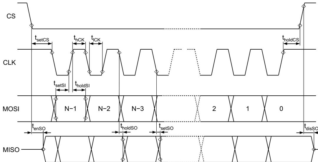
Table 7: SPI Slave Interface Timing Parameters
