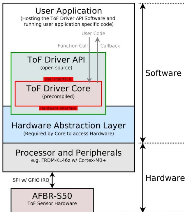
Figure 25 shows the software architecture overview for the basic implementation of the ToF driver core into user hardware and software. The precompiled core is embedded into open source API layers, providing an interface to the user application. A hardware interface declares the required hardware access for the ToF driver core to the underlying hardware and peripherals. The latter is required to connect the core to the AFBR-S50 ToF sensor hardware through the SPI and GPIO interfaces.
