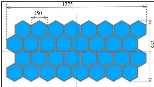
**Figure 6: Field-of-View Description of the Sensor**
