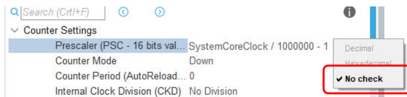
Figure 22: Disabling the Parameter Check for the Prescaler Setting
