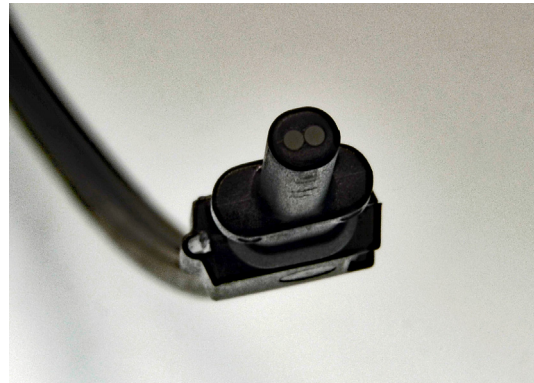
Figure 9 POF Cable Terminated with a AFBR-S10TR011Z Slim Connector
