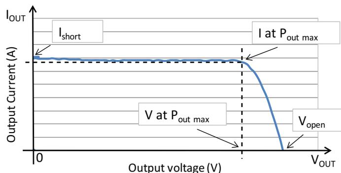
Figure 2 illustrates the typical output current vs. output voltage characteristics of an optical power converter.
