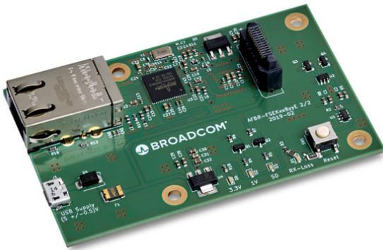
This PCB, which has been designated as board A and board D in Figure 2, is based on the chip BCM54210 from Broadcom. In the AFBR-FSEK50B00E evaluation kit, the BCM54210 chip has been configured to operate as a 1000BASE-T-to-1000BASE-X Media Converter, as shown in Figure 4.
