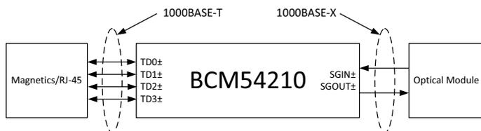
The Media Converter operation mode allows the communication between the user's application connected to the RJ-45 connector located on this PCB and the Optical Wireless Transceiver AFBR-FS50B00 located on the Optical Wireless Transceiver Front-end PCB. The device receives the data stream from the user's application through the RJ-45 port of boards A or D and delivers it to the Optical Wireless Transceiver AFBRFS50B00 of boards B or C (see
