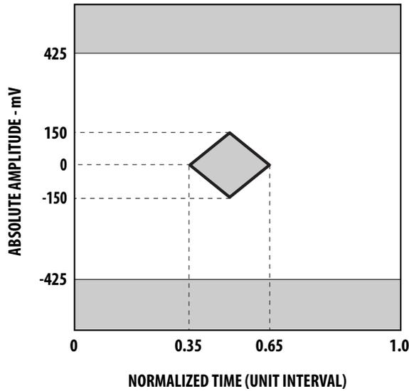
Figure 5a. Receiver Electrical Optical Eye Mask Definition
