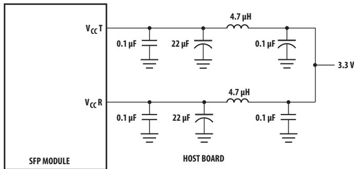
NOTE: INDUCTORS MUST HAVE LESS THAN 1Ω SERIES RESISTANCE TO LIMIT VOLTAGE DROP TO THE SFP MODULE.
