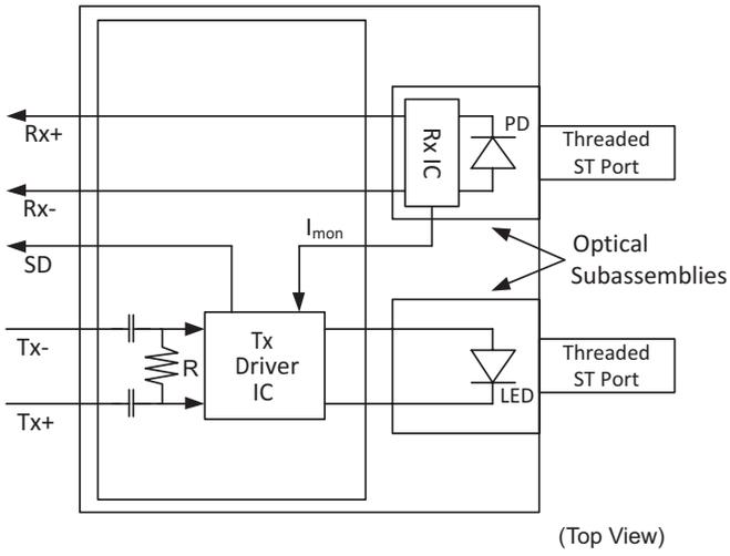
**Figure 2: Block Diagram 1 × 9 SC Transceiver**
