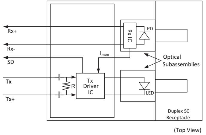
**Figure 3: Block Diagram 2 × 9 ST Transceiver**
