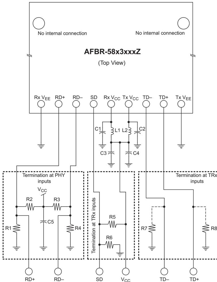
**NOTE:** The split-load termination for ECL signals needs to be located at the input of devices receiving those ECL signals. For the application board, it is recommended to use a four-layer printed circuit board with 50Ω microstrip signal paths. The value of the elements shown in the schematic in [Figure 10](#) are as follows:
