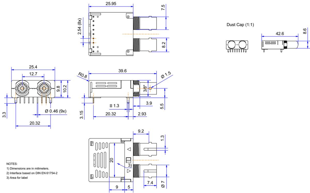
Figure 6: 2 × 9 ST Package Outline Drawings (Dimensions in mm)
