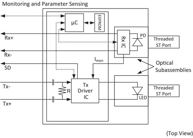
**Figure 4: Block Diagram 2 × 9 SC Transceiver**
