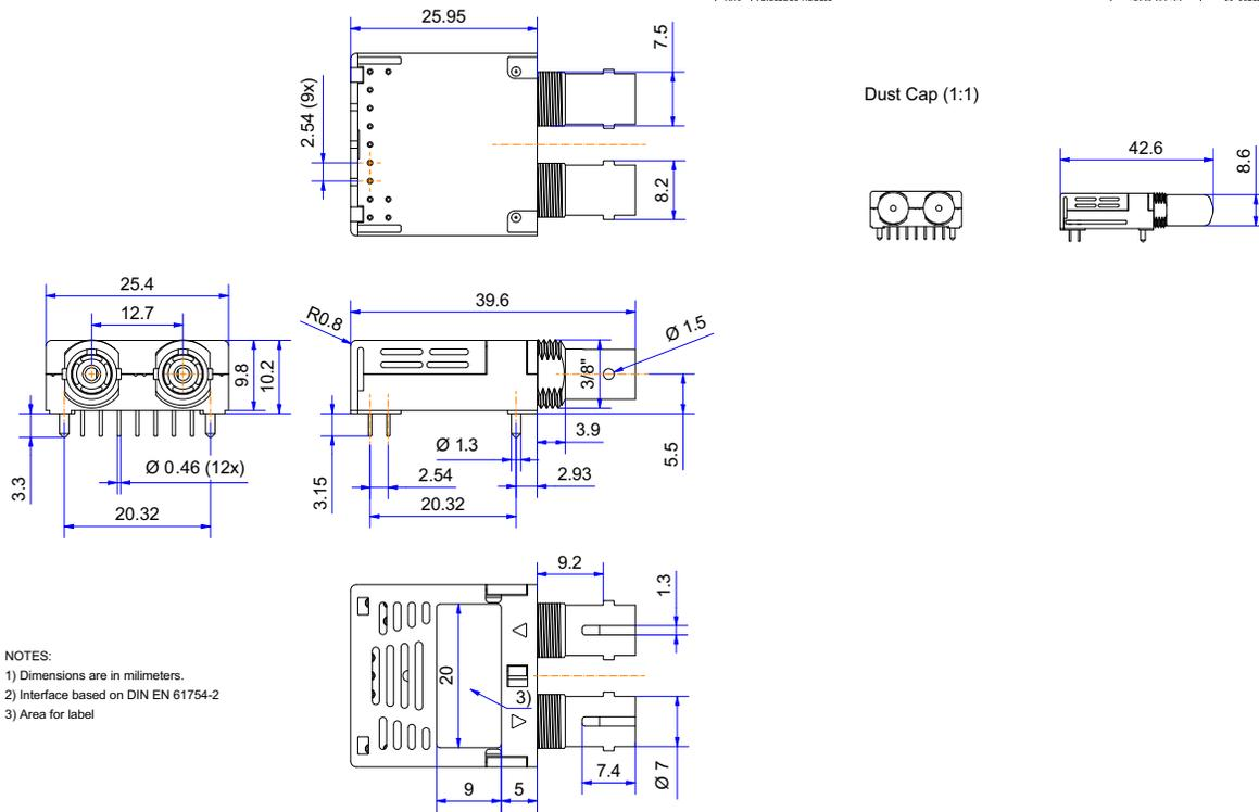
Figure 7: 1 × 9 SC Package Outline Drawings (Dimensions in mm)
