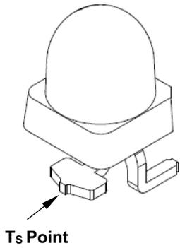
$T_S$  can be easily measured by mounting a thermocouple on the soldering joint as shown in preceding figure, while  $R_{\theta J-S}$  is provided in the data sheet. Verify the  $T_S$  of the LED in the final product to ensure that the LEDs are operating within all maximum ratings stated in the data sheet.
