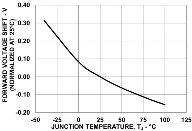
Figure 8: Forward Voltage Shift vs. Junction Temperature
