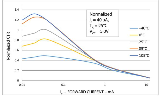
Figure 5: Current Transfer Ratio vs Forward Current
