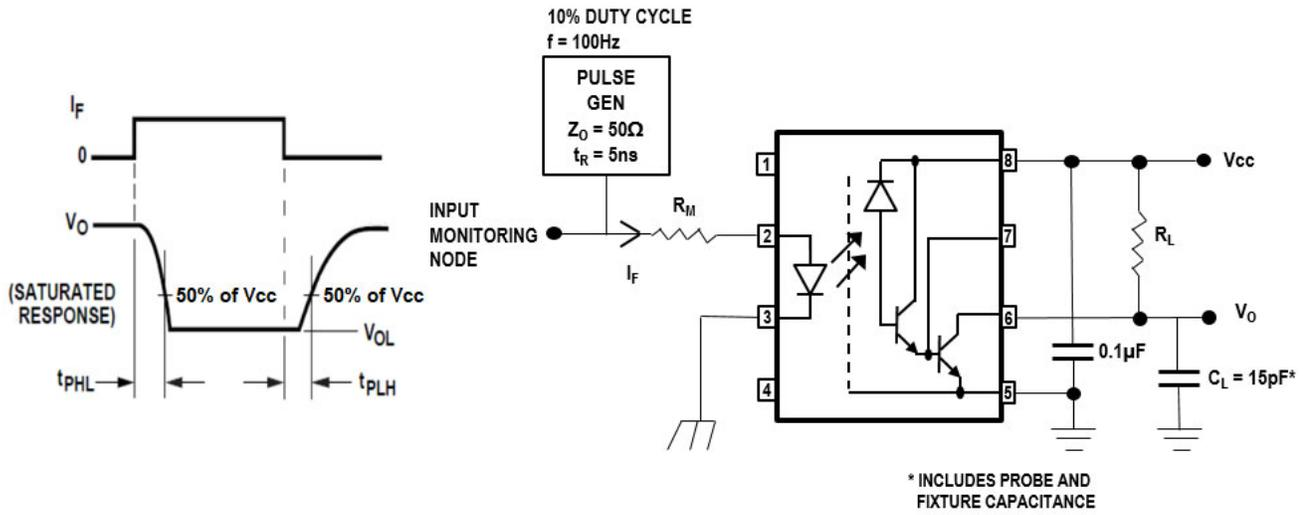
Figure 15: Test Circuit for Transient Immunity and Typical Waveforms
